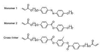
Scheme 1. Chemical structures of the two monomers and cross-linker.
