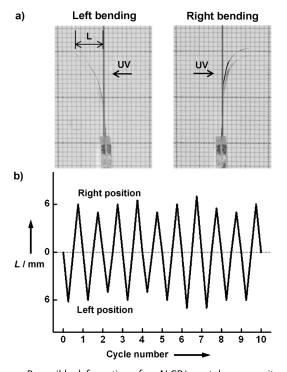
Figure 2. Reversible deformation of an ALCP/nanotube composite strip under the same UV light. a) Photographs of the tunable direction during the photomechanical deformation; b) the reversible deformation characterized by tracing the bent distance from the upright line.
