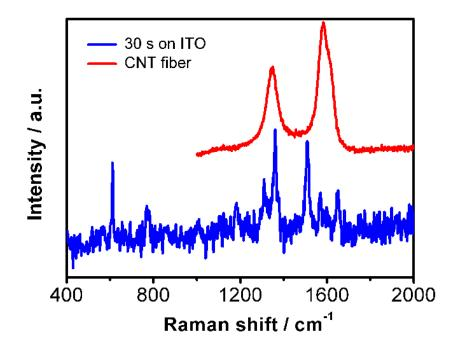
**Fig. S5** Raman spectra of a bare CNT fiber (red line) and silver nanoparticles on an ITO conductive glass after electrodeposition for 30 s (blue line).
