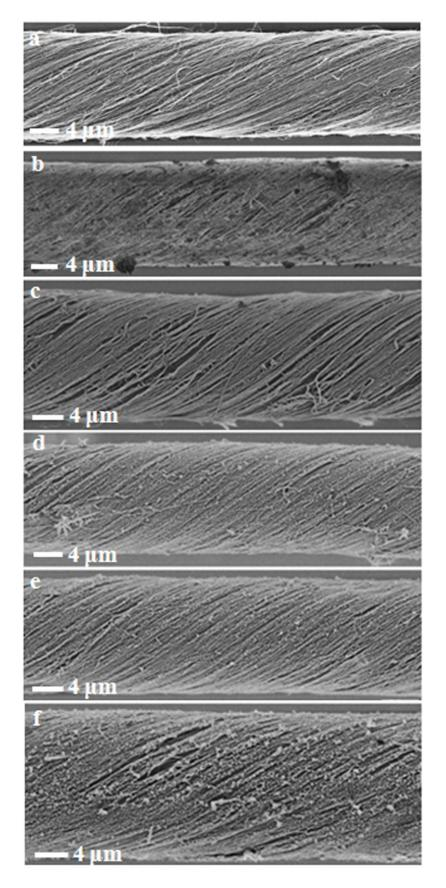
**Fig. S3** SEM images of CNT/Ag composite fibers with electrodeposition times of (a) 0s, (b) 5s, (c) 10s, (d) 30s, (e) 50s, (f) 80s.
