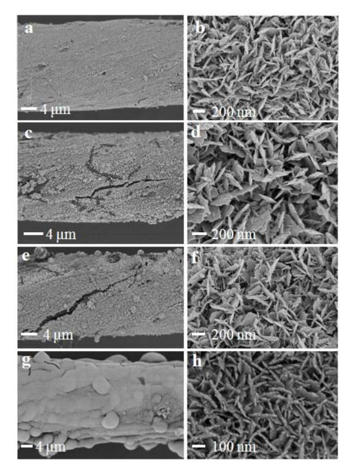
**Fig. S4** SEM images of CNT/Pt composite fibers with CV cycles of (a,b) 10, (c, d) 20, (e, f) 30, (g, h) 50.
