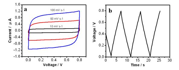
Fig. S7 (a) Cyclic voltammograms of a wire-shaped supercapacitor based on bare CNT fibers. (b) Galvanostatic charge-discharge curve measured at a current of  $1 \mu A$ .
