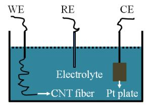
**Fig. S1** Schematic illustration for electrochemical deposition in a three-electrode system. WE, RE and CE correspond to working, reference and counter electrodes, respectively.
