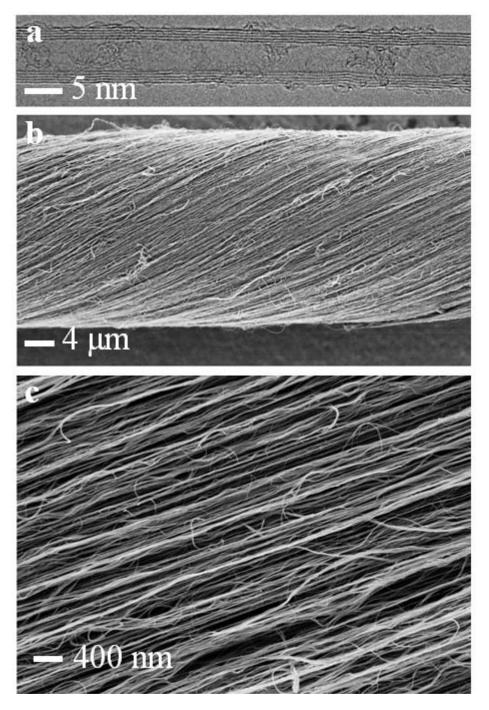
**Fig. S2** (a) Transmission electron microscopy (TEM) image of a CNT. (b, c) Scanning electron microscopy (SEM) images of a CNT fiber at low and higher magnifications.
