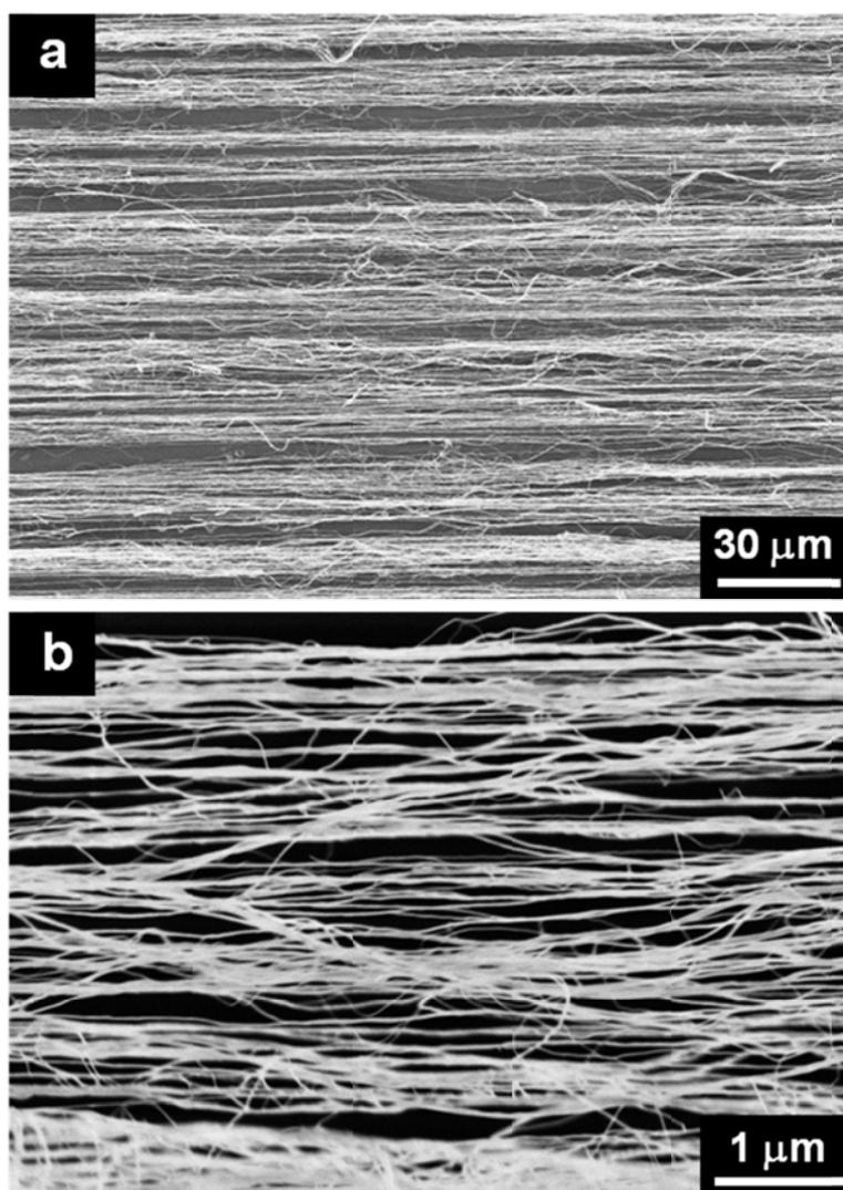
**Figure S5.** Scanning electron microscopy images of a highly aligned MWCNT sheet at (a) low and (b) high magnifications.
