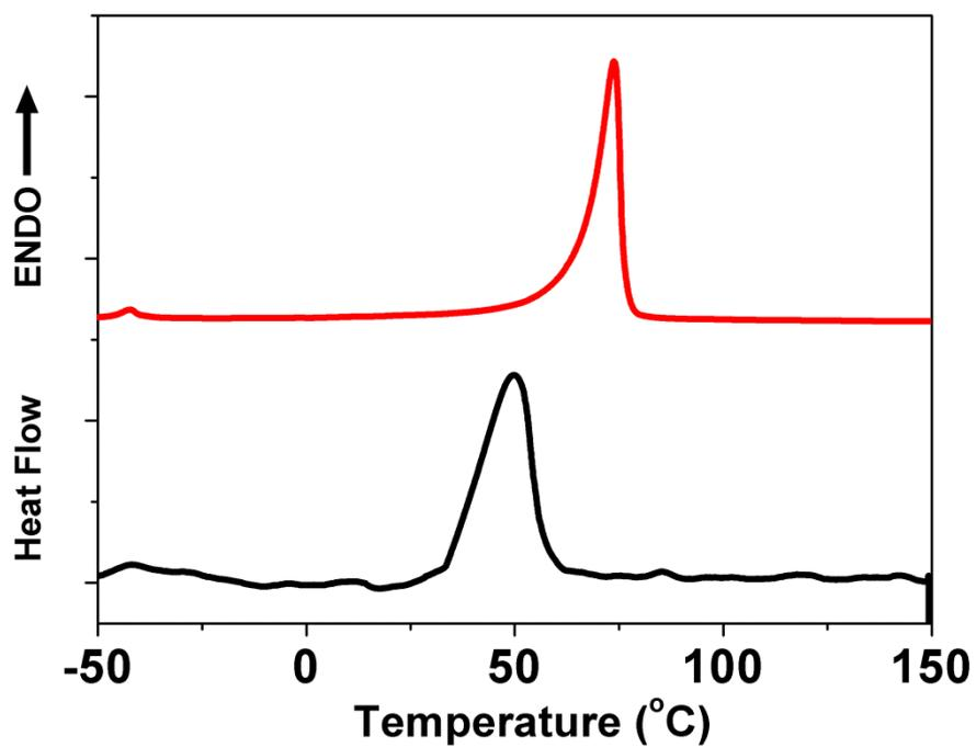
**Figure S2.** Thermal analysis of EMII (red line) and quasi-solid-state electrolyte (black line).
