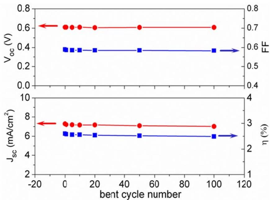
**Figure S8.** Photovoltaic parameters before and after bending for different cycles.
