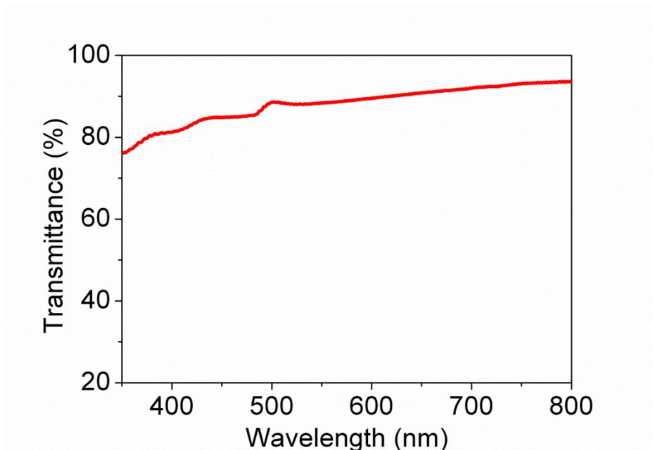
**Figure S7.** UV-vis spectra of an aligned MWCNT sheet with a thickness of 20 nm.
