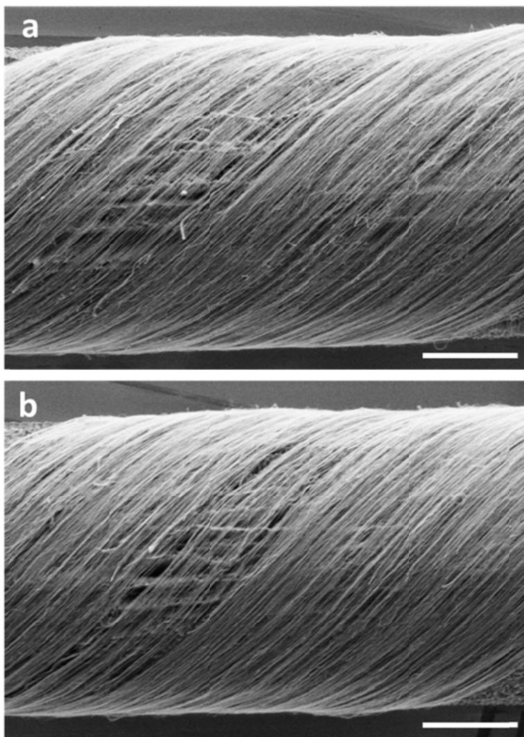
**Figure S10. a and b.** Scanning electron microscopy images of a coaxial fiber-shaped DSC before and after bending for 10 cycles, respectively. The scale bars are the same of 50 μm.
