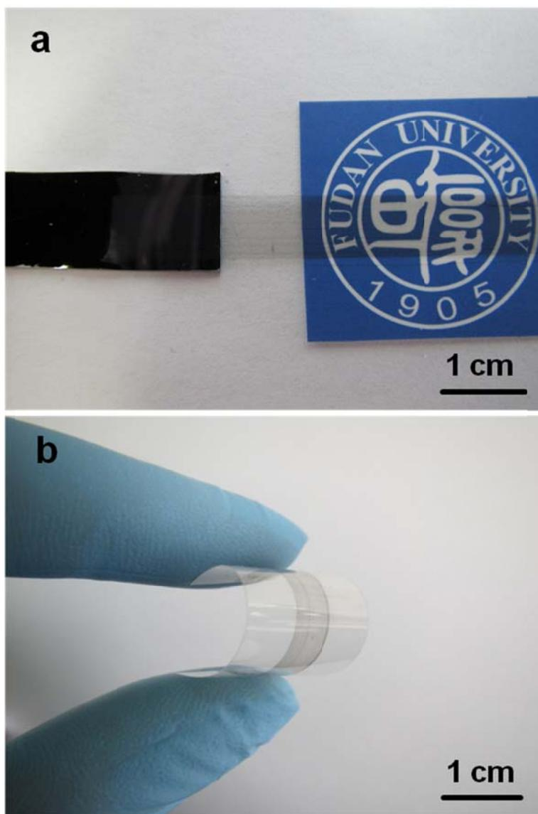
**Figure S4.** Photographs of MWCNT sheets. **a.** A single layer of MWCNT sheet with thickness of 20 nm being pulled out of a spinnable MWCNT array. The logo of Fudan University below the sheet can be clearly observed. **b.** A MWCNT sheet being attached on a flexible and transparent polyethylene terephthalate film.
