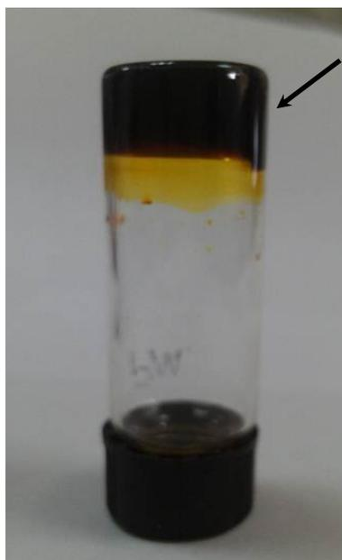
**Figure S3.** Photograph of the electrolyte in an inverted bottle. The arrow shows the quasi-solid-state electrolyte.
