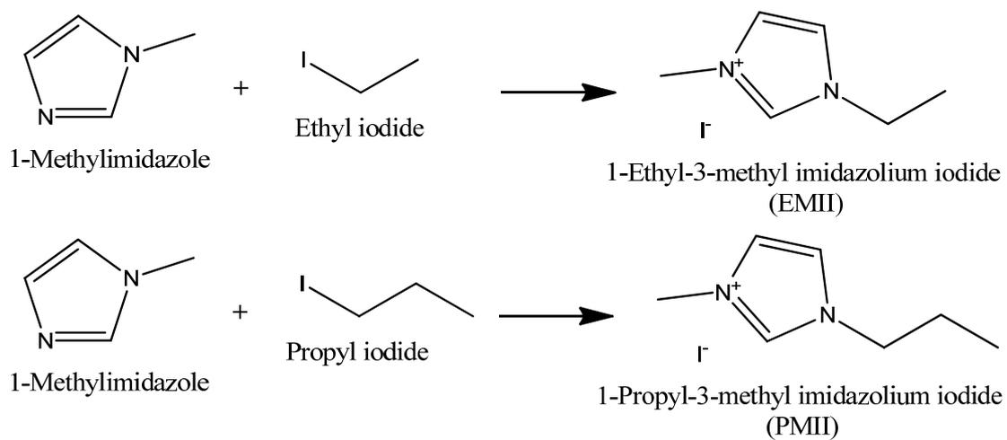
**Figure S1.** Schematic illustration to the synthesis of the ionic liquid crystal of 1-ethyl-3-methylimidazolium iodide (EMII) and ion liquid of 1-propyl-3-methylimidazolium iodide (PMII).
