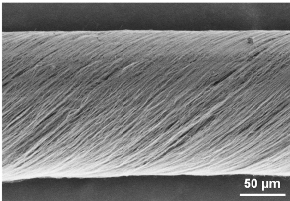
**Figure S6.** Scanning electron microscopy image of a MWCNT sheet with thickness of 60 nm being wrapped on a titania nanotube-modified Ti wire.
