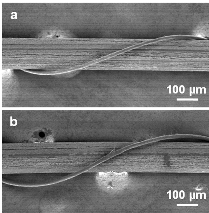
**Figure S9. a and b.** Scanning electron microscopy images of a twisted wire-shaped DSC before and after bending for 10 cycles, respectively.
