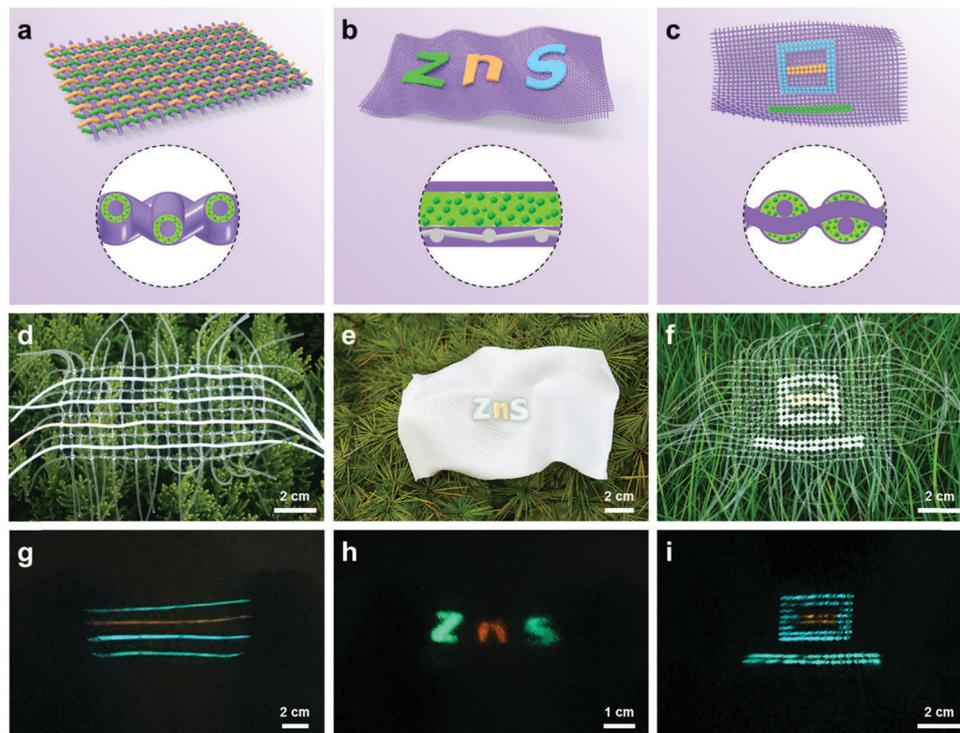
Fig. 4 Mechanoluminescent fabrics. Schematic illustrations with the structure of the mechanoluminescent fabrics based on mechanoluminescent fibers (a), ribbons (b) and dots (c); (d–f) photographs of the mechanoluminescent fabrics based on mechanoluminescent fibers (d), ribbons (e) and dots (f); (g–i) photographs of the mechanoluminescent fabrics shown in (d–f) during the stretch and release process.
