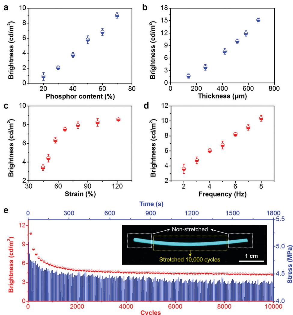
**Fig. 2** Mechanoluminescence measurements. Dependence of the mechanoluminescence intensity of the composite fiber on phosphor content (a), thickness of the mechanoluminescent layer (b), strain (c) and frequency (d); (e) evolution of the mechanoluminescence intensity (red) and mechanical strength (blue) of the composite fiber during stretch and release cycles (inset, photograph of the composite fiber under UV irradiation after 10 000 cycles of stretch and release).
