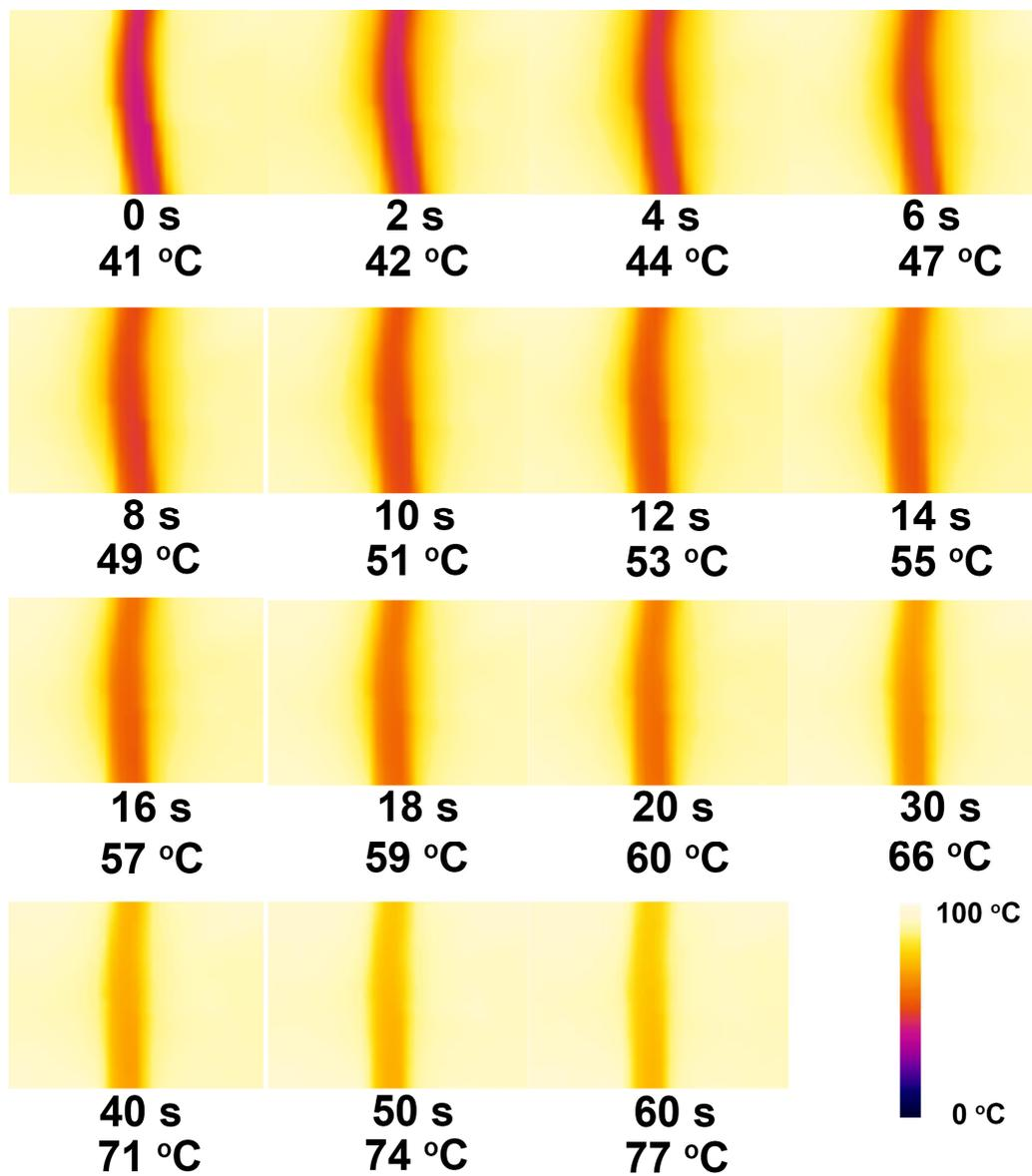
**Figure S4.** Thermographs of the lithium-air battery under heating.
