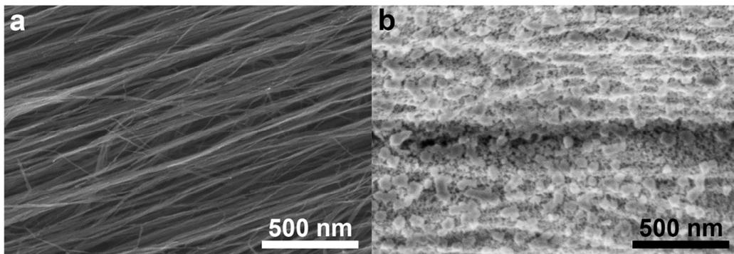
**Figure S1.** SEM images of the CNT sheets of a) pristine and b) discharged cathode.
