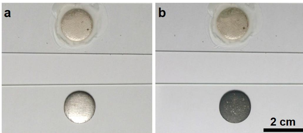
**Figure S10.** Photographs of a Li foil with (top) and without (down) the coat of ionic liquid gel electrolyte a) before and b) after exposure in air for 30 min.
