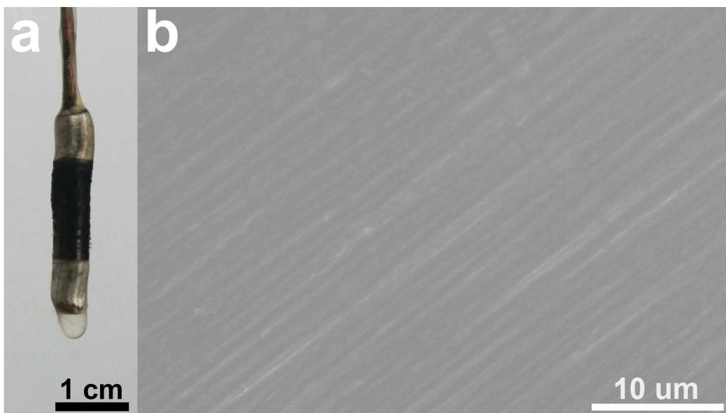
**Figure S9.** a) Photograph of the aligned CNT sheet-wrapped lithium-air battery and b) SEM image of the surface of the aligned CNT sheet.
