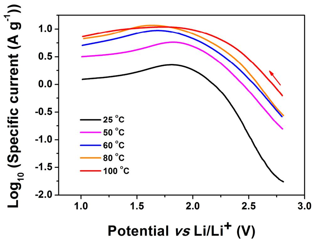
**Figure S6.** Tafel plots of the air electrode (cathode) at different temperatures during the reduction reaction ( $\text{Li/Li}^+$  used as counter and reference electrode).
