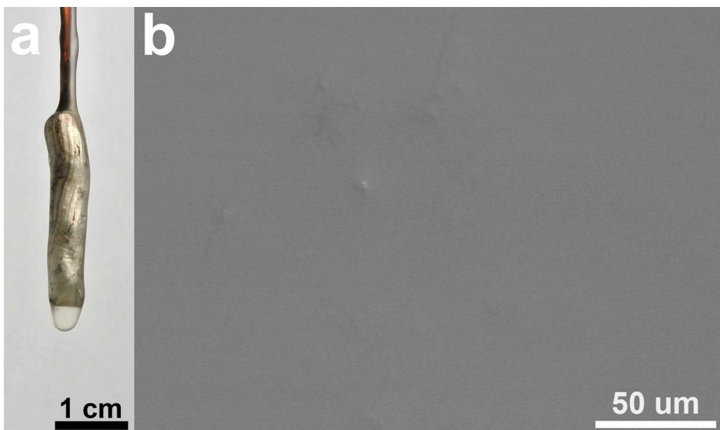
**Figure S8.** a) Photograph of the ionic liquid gel electrolyte covering on a lithium wire and b) SEM image of the gel electrolyte.
