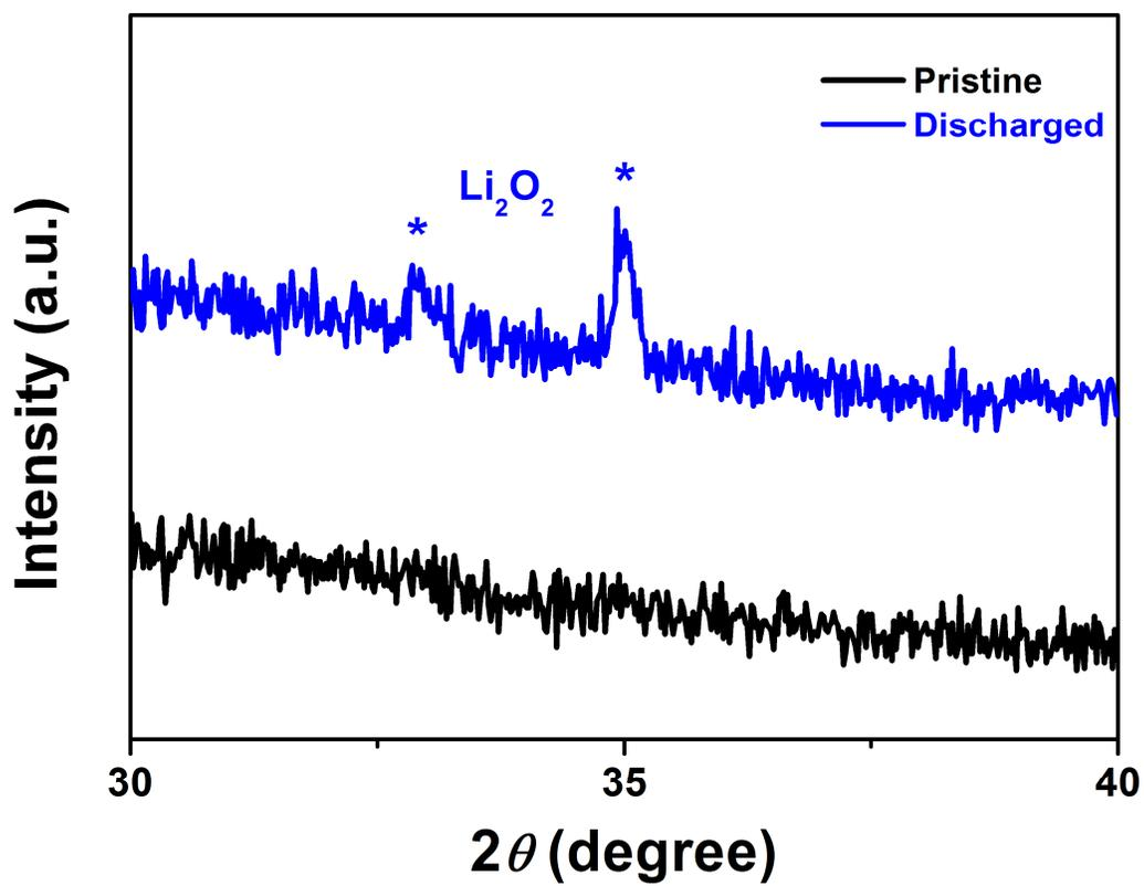
Figure S2. XRD patterns of the pristine and discharged cathode.
