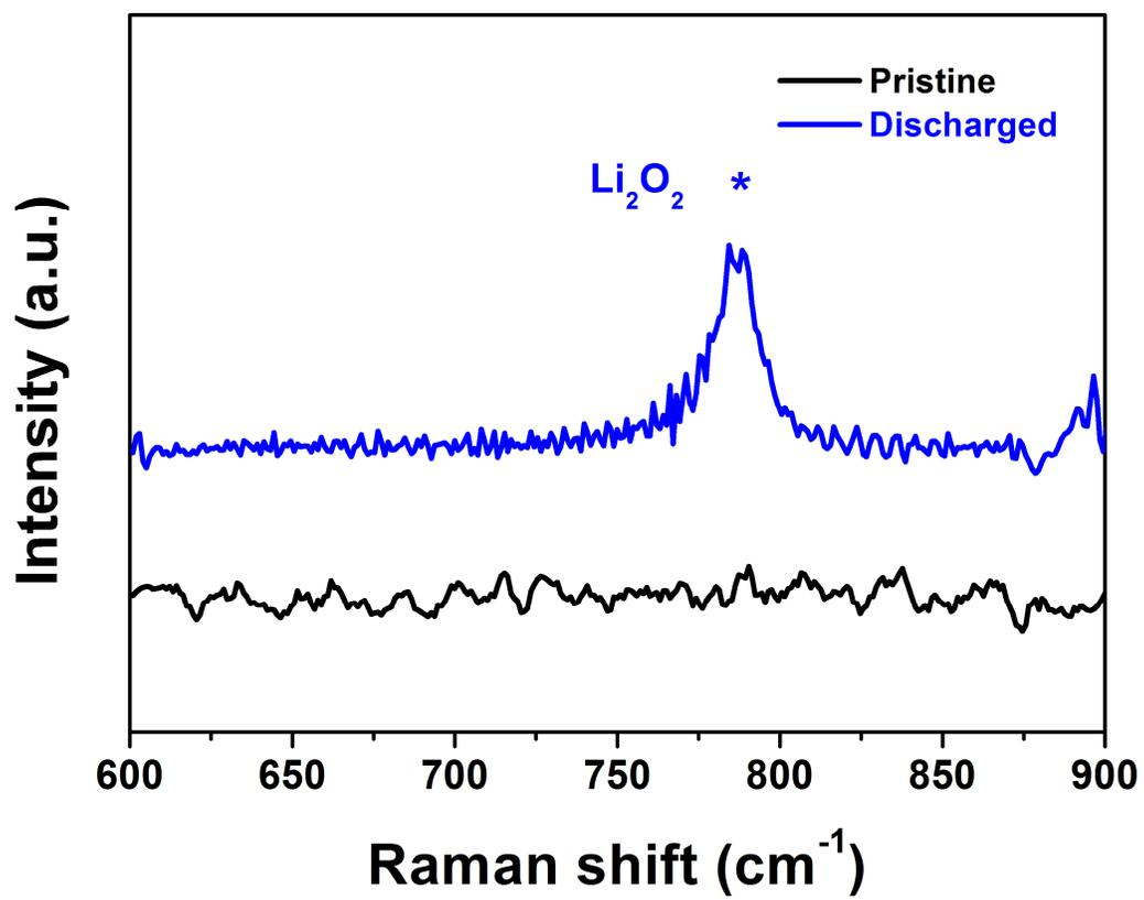
Figure S3. Raman spectra of the pristine and discharged cathode.
