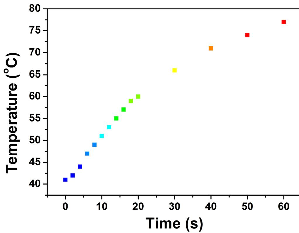
**Figure S5.** The temperature increase of the lithium-air battery during heating.
