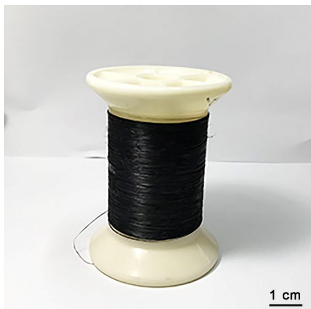
Figure S1. Photograph of a roll of CNT fiber.
