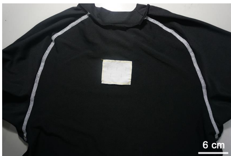
Figure S14. Photograph of a garment device embedded with sensing fiber units knitted into the fabric.
