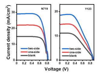
Figure S6. J-V curves of N719 and Y123 based FDSSCs, one-side attached, and two-side
