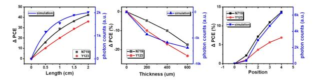
Figure S7. Experimental PCE and simulated photon number variation of FDSSCs with (a) side-attached, (b) top-covered, and (c) bottom-attached LSCs.
