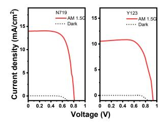
Figure S5. Dark current of the N719 and Y123 FDSSCs.
