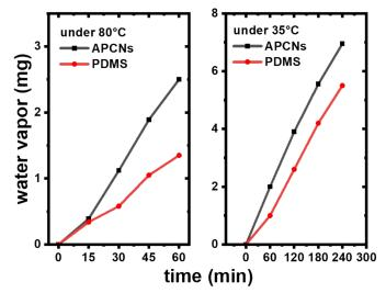
Figure S3. Water vapor permeation comparison between APCNs and PDMS.
