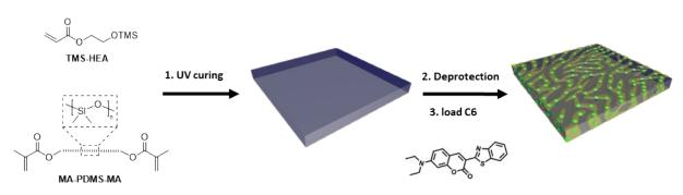
Figure S2. Synthesis scheme of APCNs containing C6.
