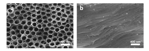
Figure S1. SEM images of (a) TiO<sub>2</sub> nanotube arrays and (b) CNT fiber surface morphology.
