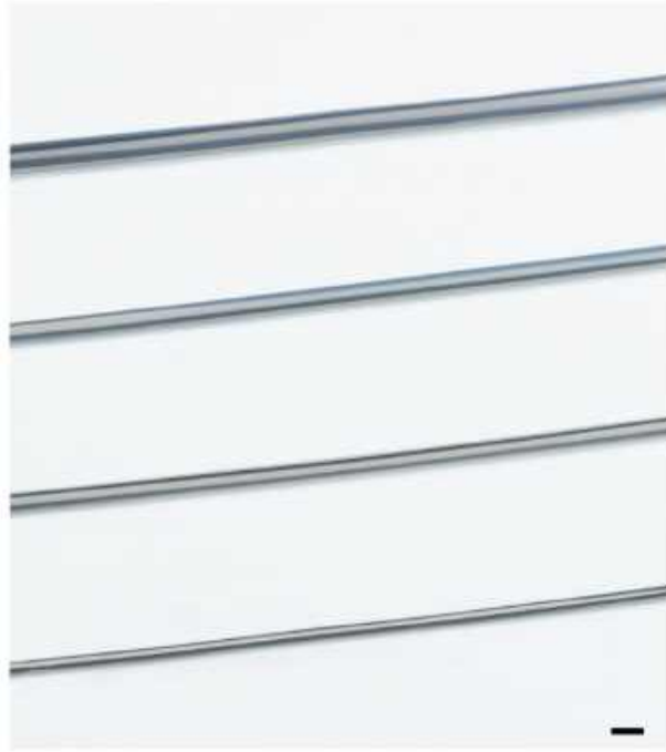
Supplementary Fig. 17 | Photograph of extruded fibre batteries with increasing diameters. Scale bar, 500 \mu\text{m} .
