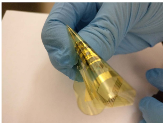
Figure 10. A fully flexible standalone integrated silicon electronic system with microprocessor, memory, BLE transceiver, antenna, an array of micro lithium ion batteries, solar cells and sensors with light actuator.
