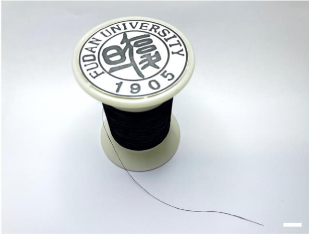
Figure S1. a) Photograph of a roll of CNT fiber. b) Photograph of a CNT fiber in the shape of treble clef. Scale bar, a) 1 cm; b) 0.5 cm.
