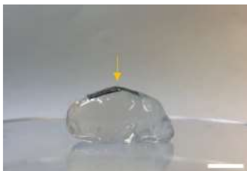
Figure S8. Photograph of FME attached to a rat brain model prepared from 0.6 wt% agar. The yellow arrow points to the location of FME. Scale bar: 1 cm.
