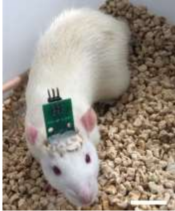
Figure S29. Photograph of a rat with FME implanted on the cerebral cortex. Scale bar: 3 cm.
