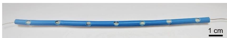
Fig. S24. Photograph of the SCL/Na–air fiber battery that exhibited a typical diameter of ~0.5 cm and a length of ~15 cm.
