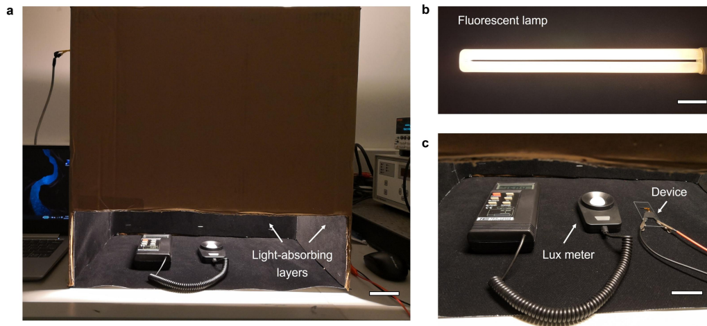
Figure S8. a) Photograph illustrating the test condition for IPVFs. Scale bar, 5 cm. The photovoltaic performances of IPVFs were measured in a specialized black box fully covered with black light-absorbing layers that could avoid the influence of reflected and scattered light on device. b) Photograph of the light source in the black box. Scale bar, 5 cm. A fluorescent lamp was used. c) Photograph illustrating the test procedure. Scale bar, 1 cm. A lux meter was used to precisely calibrate the illumination on the measured device. In the test, completely lighttight tapes were tightly covered on the needless part of the fiber photovoltaic device as a mask to precisely control the effective illumination area.
