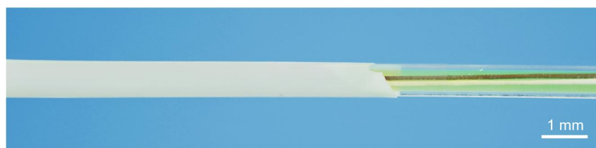
Figure S2. Photograph of the FDSSC partly covered with light diffusion layer. The light diffusion layer gives the solar cell a white appearance, which can effectively hide the internal electrode structure and achieve visual integration.
