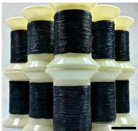
Figure S1. Photograph showing rolls of continuous CNT sheets. Scale bar, 2 cm.
