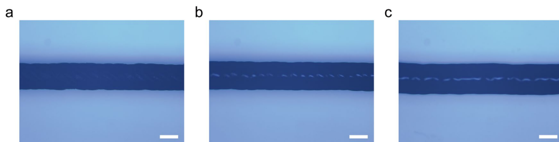
Figure S4. Optical micrographs of fiber BSC electrodes a) before PVA coating, b) coated with PVA once and c) coated with PVA for three times. The thicknesses of PVA layer were about 6 and 20 \mu\text{m} in (b) and (c), respectively. Scale bar, 200 \mu\text{m} .
