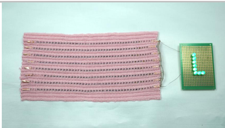
Figure S22. An FLIB textile consisting of eight 0.2-m-long LCOIBFCC-G FLIBs to power light-emitting devices. The FLIB textile size was about 0.2 m×0.1 m.
