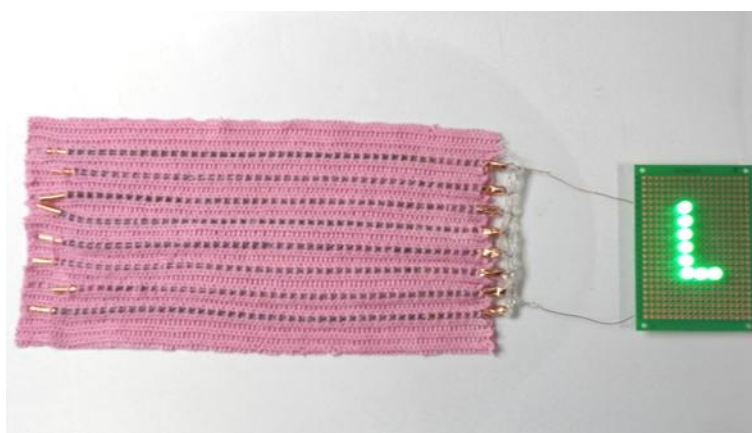
Figure S23. The soaked textile battery as shown in Figure 4h powering light-emitting diodes after wringing out the water.
