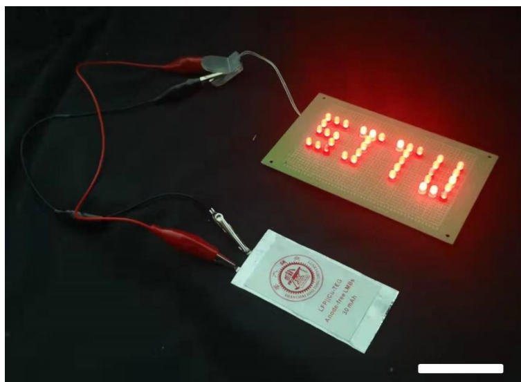
Fig. S32. An anode-free pouch cell readily lightening up an LED array comprised of 37 in-parallel LED lamps. Scale bar, 5 cm.
